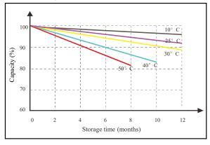
Note 2: The above curves are based on laboratory testing data @  $25^{\circ}\text{C}$  40%RH.
